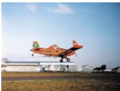
Ethanol from sugarcane powers the single-seat EMB 202 Ipanema for farm use.
