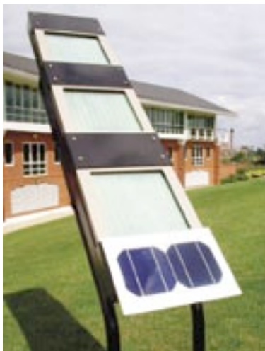
A novel type of solar cell, which has been crafted into array panels, produces hydrogen rather than electricity.
