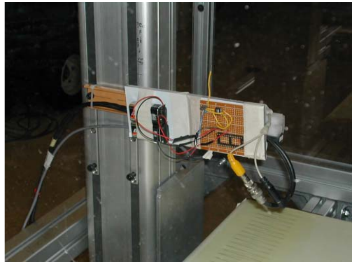
Figure 6. Ion detector mounted to the Robo-moth gantry
